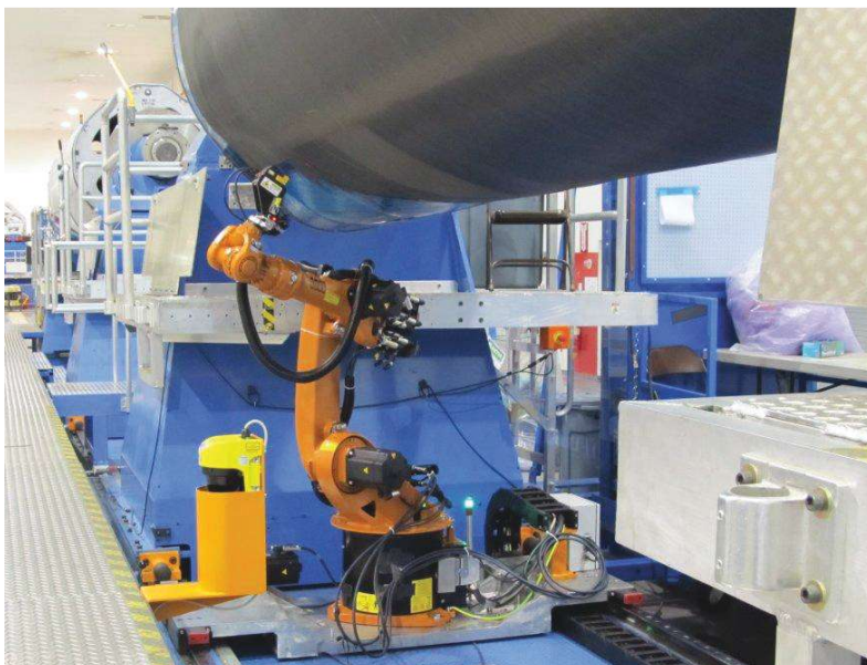
FIG. 3 ACSIS in-process inspection
