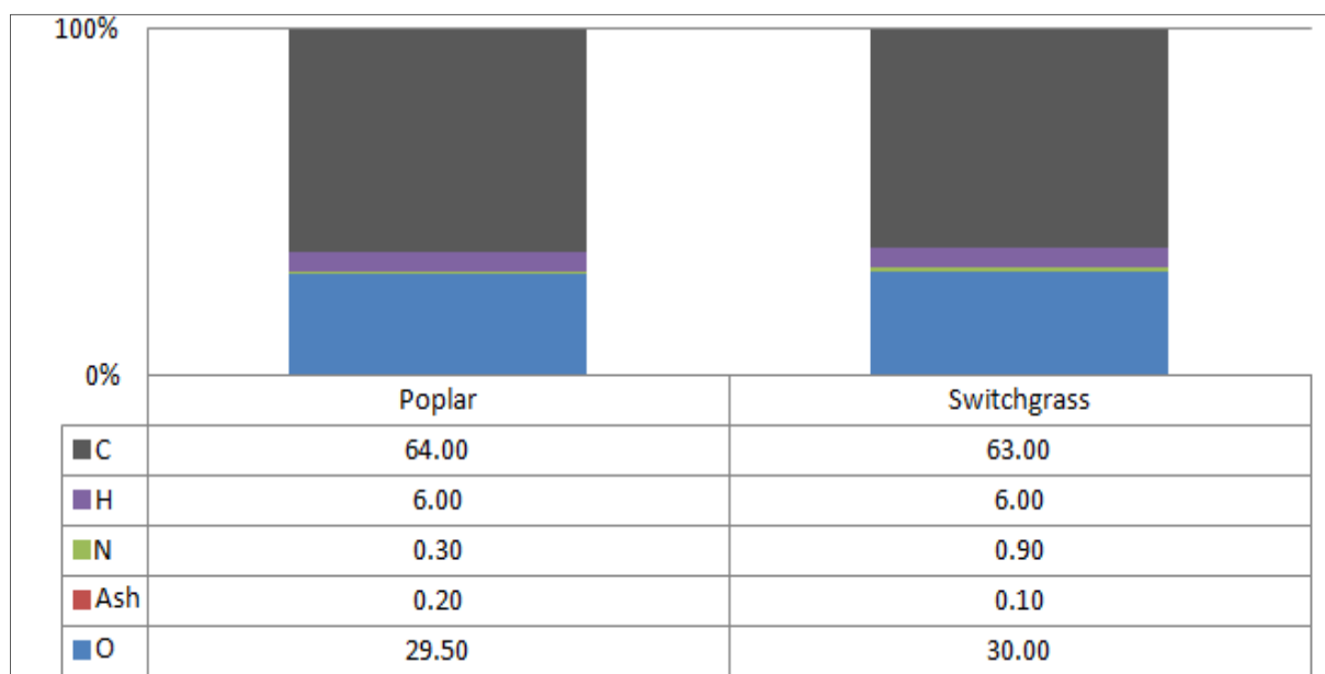
Figure 36. Elemental analysis of poplar and switchgrass showing carbon, hydrogen, nitrogen, ash and oxygen content.
